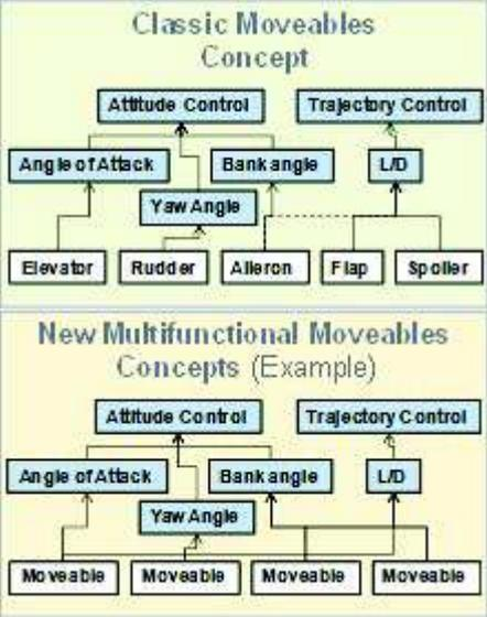
**Fig 13 : Principle of the functional driven moveables approach**
