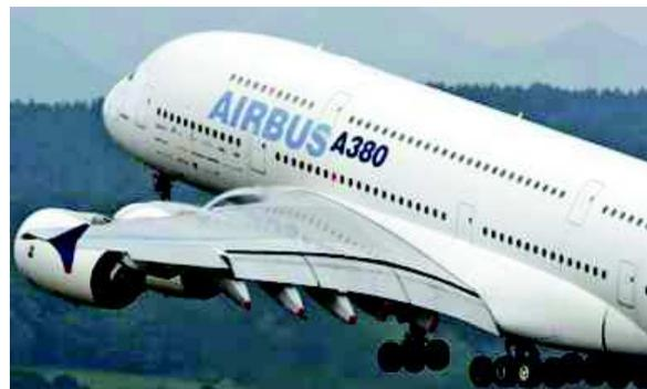
**Fig 1: Airbus A380 in high-lift configuration**
