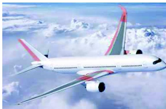
**Fig 16: Local active separation control – potential areas of application on future transport aircraft configurations (in red)**
