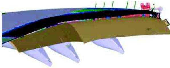
**Fig.11: Flap, spoiler and support station layout of the Adaptive Dropped Hinge Flap**
