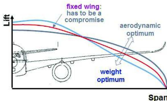
**Fig 10: Spanwise load control with variable camber & differential flap setting**
