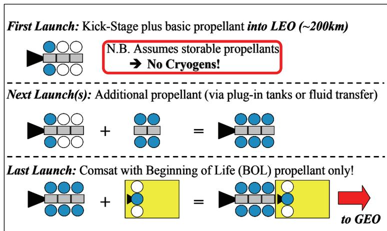
because all have a beginning of life (BoL) mass ~35% below their initial launch mass. This is because a significant fraction of their launch mass is propellant that they must burn in order to transfer themselves from GTO to GEO. The key to servicing these markets is, therefore, the on-orbit assembly of a kick-stage capable of delivering the comsat directly into GEO, as illustrated in Figure 7.
